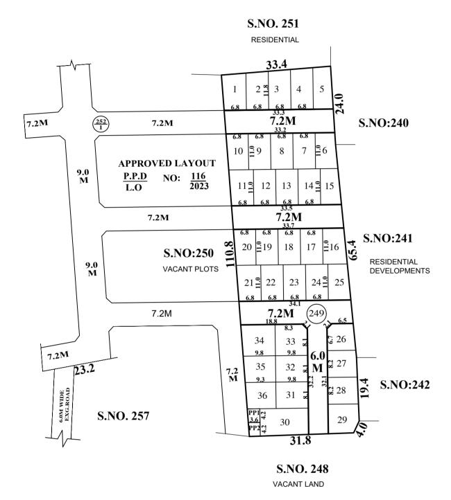
SITE EXTENT (AS PER PATTA) **3600 SO.M** ROAD AREA 932 SQ.M PUBLIC PURPOSE PROVIDED (1%) PP-1 HANDED OVER TO THE LOCAL BODY (0.5%): 15.5 SQ.M PP-2 HANDED OVER TO THE TANGEDCO (0.5%): 14.5 SQ.M NO. OF PLOTS 1. SPLAY - 1.5M x 1.5M 2. MEASUREMENTS ARE INDICATED EXCLUDING SPLAY DIMENSIONS 3. ROAD AREA WERE HANDED OVER TO THE LOCAL BODY VIDE GIFT DEED **PUBLIC PURPOSE-1** PUBLIC PURPOSE-2 DOC.NO:6357/2023, DATED:15.07.2023 @ SRO,PAMMAL (RESERVED FOR TANGEDCO)
